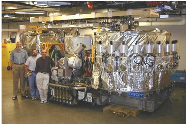
Fig. 1. The superconducting electron storage ring Helios-1 at Jefferson Lab. The synchrotron radiation ports are sealed by valves and can be seen on the right of the photo. L – R. Andrew Hutton, Ron Lauzé and Gwyn Williams.
