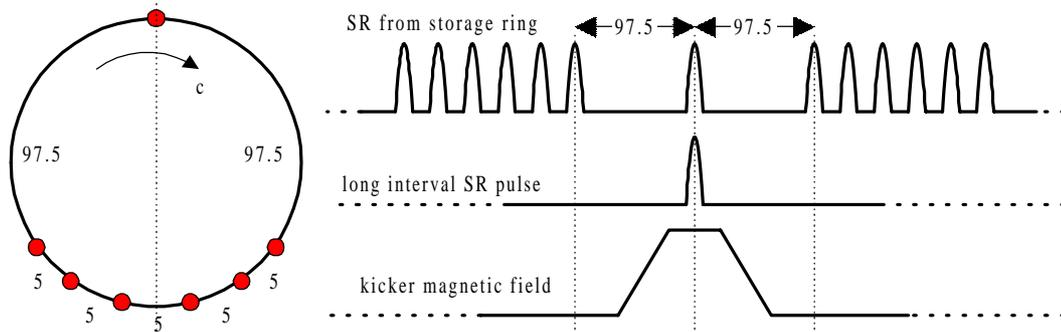
Fig.9. Electron bunches in storage ring with asymmetry ( reference coordinate: time ns )
