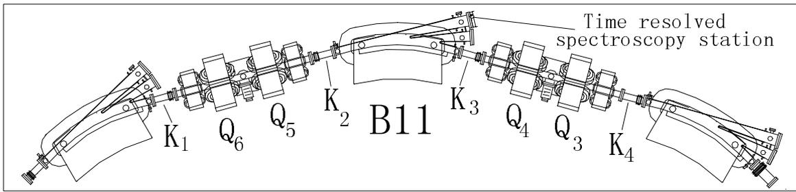
Figure 3: Layout of storage ring at bump area
