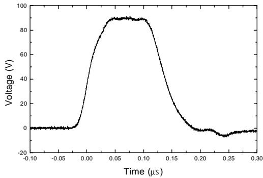
Fig.8 Waveform of discharge current(950A)
