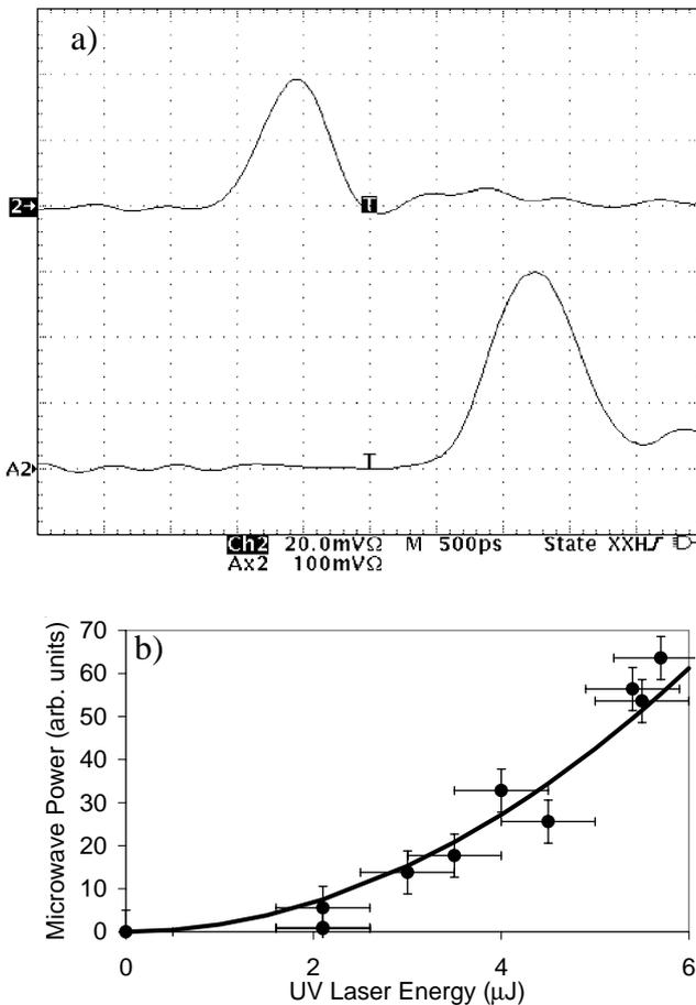
Figure 2: a) Upper trace: x-band detector signal, Lower trace: laser photodiode signal. Both are at the resolution of the detectors. b). Microwave power as a function of laser energy with a quadratic fit.
