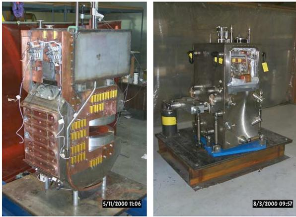
Figure 3: First magnet/cryostat assembly.
