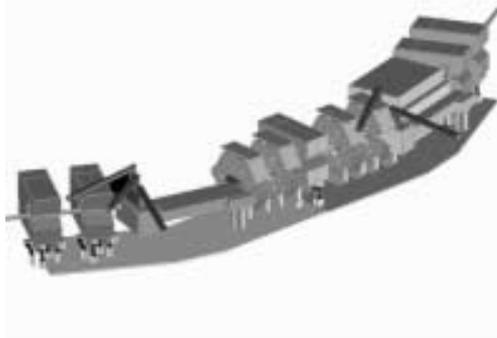
Figure 2: Conceptual view of ring arc sector. IR light ports are extracted from the end of each dipole vacuum chamber.
