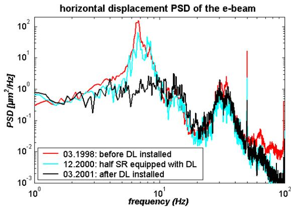
Figure 3: Horizontal displacement PSD of the electron beam before, during and after the installation of the damping links in the storage ring.
