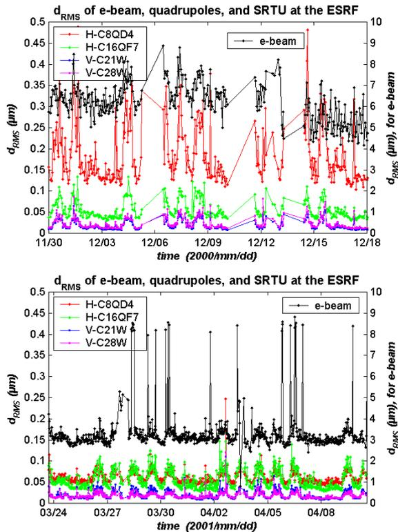
Figure 1: RMS displacement in the frequency range of 4-12 Hz of the e-beam, quadrupoles and SRTU wall versus time.
