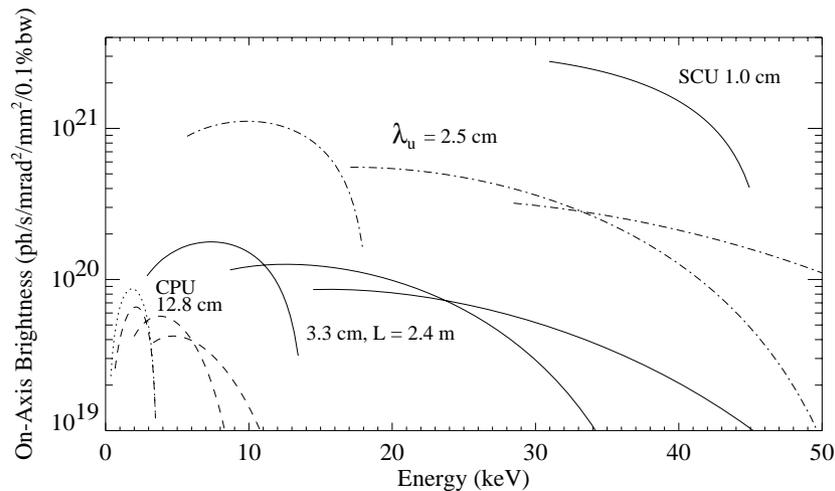
Figure 2: On-axis brightness for a future APS low- $\epsilon_x$  (3.6 nm-rad) low- $\epsilon_y/\epsilon_x$  (0.25%) lattice at 7.0 GeV and 300 mA with 7.7-m-long undulators. For the 3.3-cm-period undulator A the performance is for a 2.4-m-long device. For the CPU, both the circular (dots) and linear (dashes) polarization modes are shown. The SCU is a proposed superconducting undulator.
