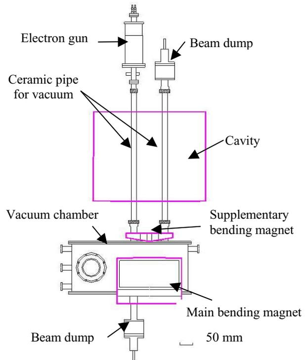
Fig. 1. Schematic diagram of acceleration system
