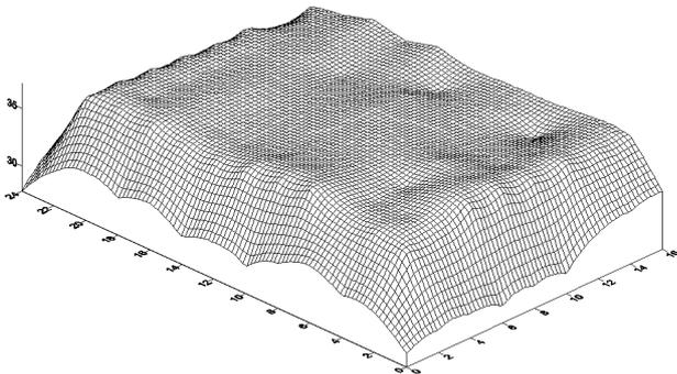
Fig. 5. Measured magnetic flux density profile
