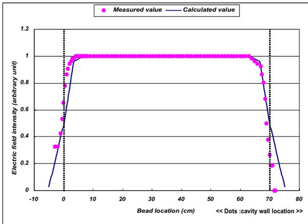
Fig. 2. Electric field distribution along the beam hole
