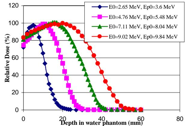
Figure 3: Measured dose penetration depth curves in water phantom for the IORT-1 system
