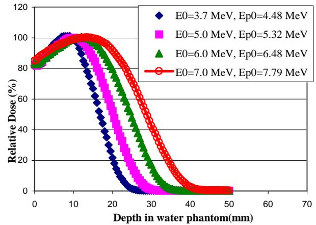
Figure 2: Measured dose penetration depth curves in water phantom for the NOVAC7 system
