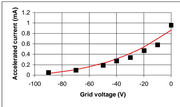
Figure 1: Measured variation of output beam current vs grid voltage: ■ measured data, — computed curve
