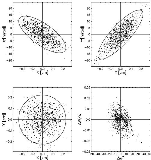
Figure 4: Particle distribution at the exit of the RFQ.
