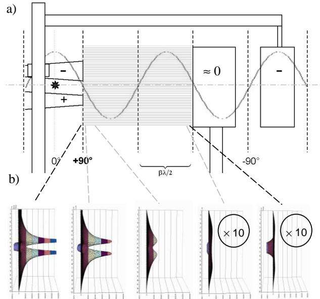
Figure 5: a) Area of interest (shaded) and its boundary conditions: -10 resp. 60 kV electrode voltage, -1,2 kV at the first drift tube (calculated by MAFIA), b) generated static potential in different planes (factorized by 10 in the last two planes).
