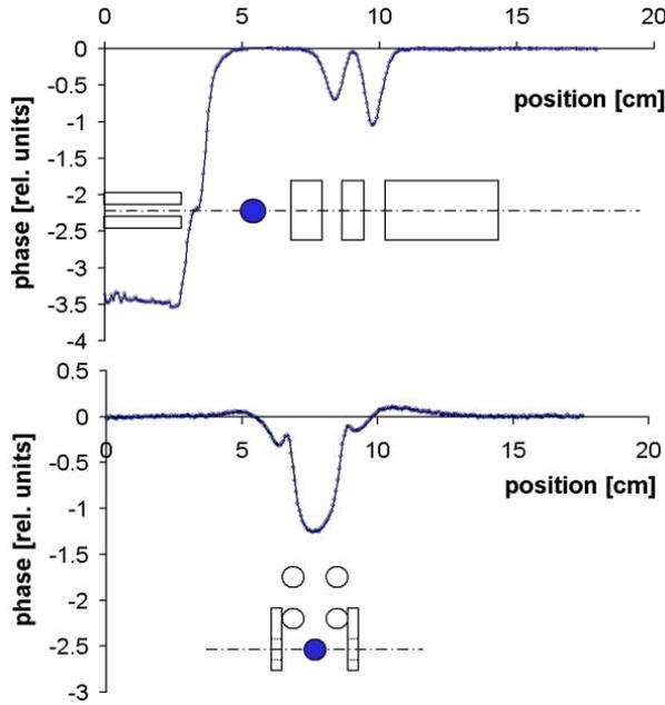
Figure 7: Bead-perturbation measurements on the model set up to compare the electrode with the buncher voltage.
