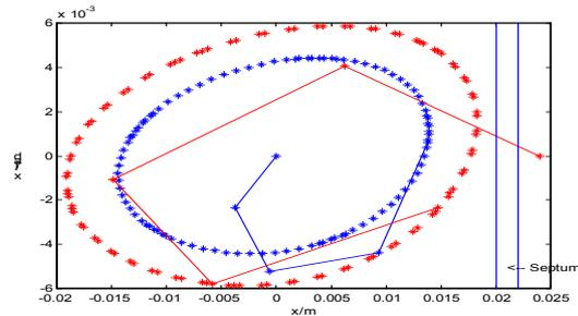
Figure 4: Injected and stored beams at the septum
