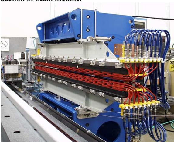
Fig. 1: View of CPU on the measurement bench.
