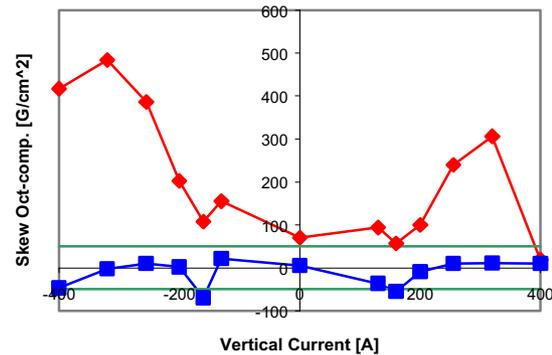
Fig. 7: Vertical current dependence of skew octupole component. Red diamonds correspond to the field components before correction. Blue squares correspond to those after correction. Green lines stand for the tolerance of the ring.
