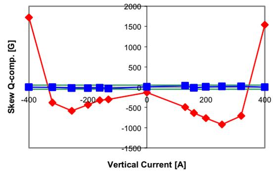
Fig. 6: Vertical current dependence of skew quadrupole component. Red diamonds correspond to the field components before correction. Blue squares correspond to those after correction. Green lines stand for the tolerance of the ring.
