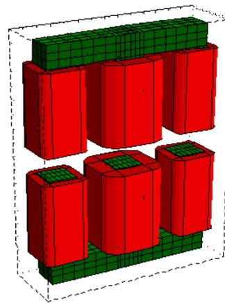
Fig. 2: Skew Quadrupole Corrector.
