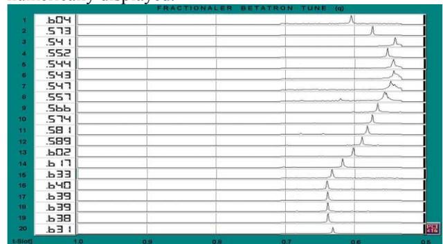
Figure 4: Display of a tune measurement in the ramp consisting of averaged FFT spectra.
