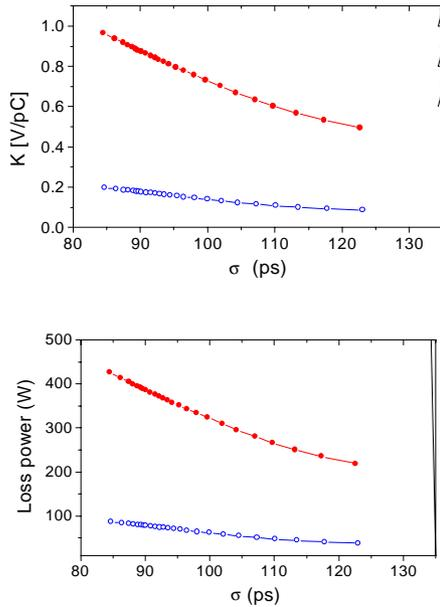
Fig2.  $K$ - $\sigma$  curves and loss power of ceramic chamber with and without coating
