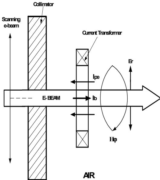
Figure 2: Electrical circuit for beam current measurements by current transformer in air:  $I_b$  is beam current and  $I_{pe}$  is current of plasma electrons.
