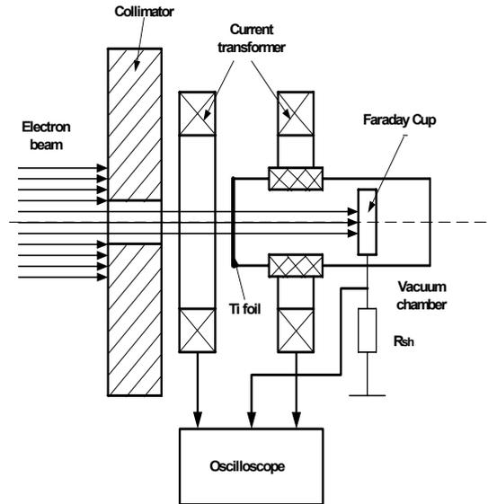
Figure 3: Block diagram of experiments.
