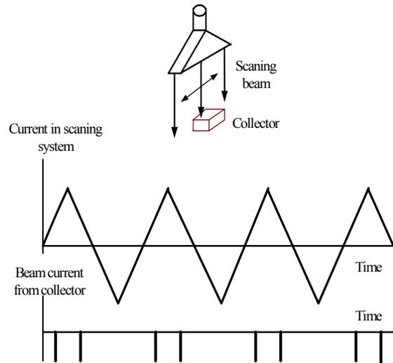
Figure 1. Pulsed mode of scanning electron beam.
