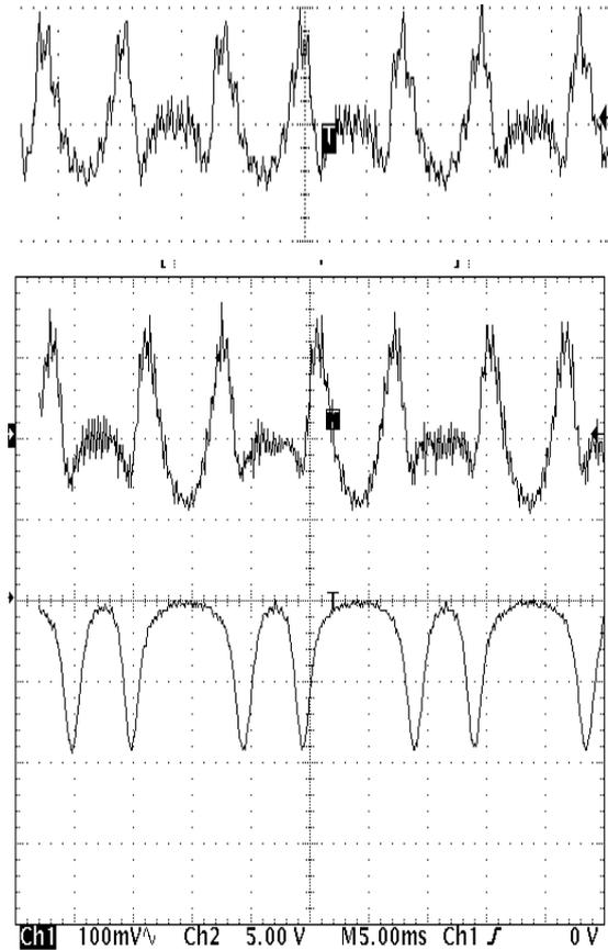
Figure 4: Typical oscillograms from current transformers in air (top) and in vacuum (middle), and from a Faraday cup in vacuum (bottom).
