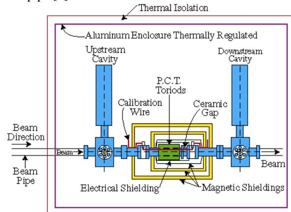
Figure 1. Current Monitor components on the beam line
