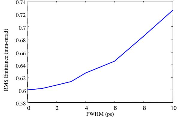
Figure 3: HOMDYN simulation of emittance vs bunch length. Charge is fixed at 2 pC, peak cathode field is 95 MV/m.
