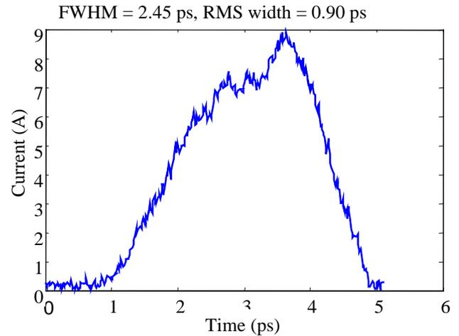
Figure 4: Time profile of electron beam using RF-zero phasing method at 75 MeV. Electron beam is transported to end of linac for this measurement.
