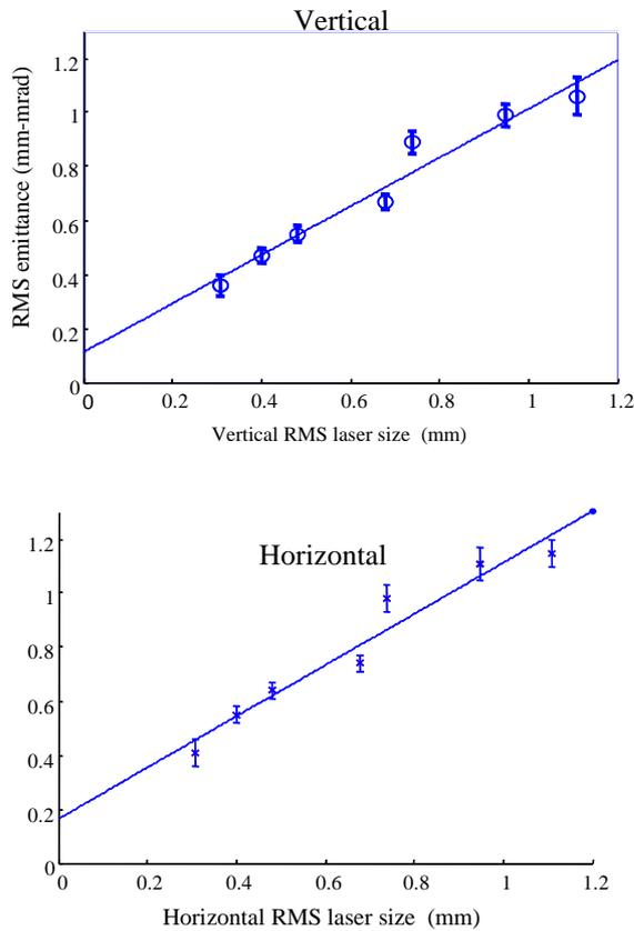
Figure 5: Plots of emittance vs RMS laser size showing linear dependence.
