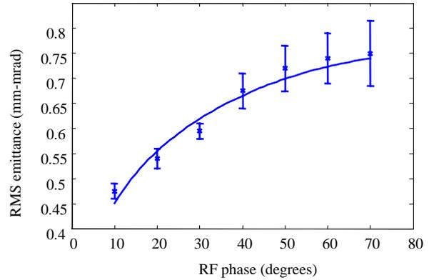
Figure 6: Data points are average of horizontal and vertical emittance plotted vs laser arrival phase at the cathode. Curve is fit using Eq.'s 2 and 3. Charge = 2 pC, FWHM = 2.5 ps, RMS laser size = 0.7 mm.
