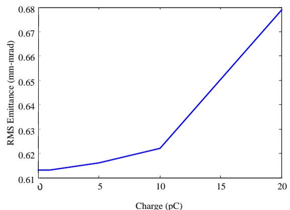
Figure 1: HOMDYN simulation showing scaling of emittance with beam charge. The initial, uncorrelated, normalized emittance is 0.60 mm-mrad. Bunch length is held fixed at 3 ps FWHM.
