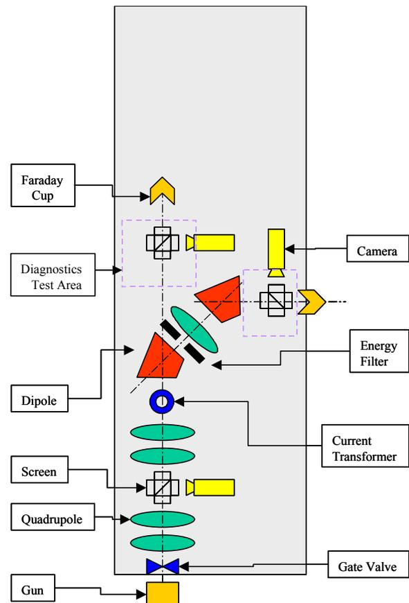
Figure 1: Injector test stand schematic beamline layout for the main injector test line.
