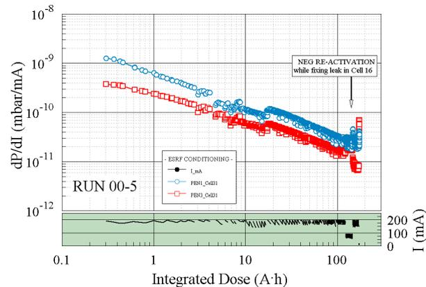
Figure 5: ESRF: Conditioning of cell 31's ID chamber. PEN1: entrance of ID chamber; PEN3: exit .
