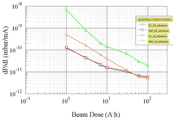
Figure 7: The Al ID chamber, void of distributed pumping and without NEG-coating, shows the longest conditioning time.
