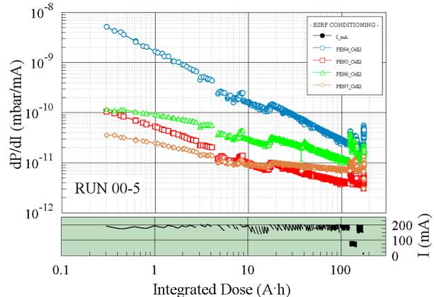
Figure 4: ESRF: Conditioning of cell 2. PEN4: entrance of dipole1, location of new BPM chamber; PEN5: on crotch 1; PEN6: entrance of dipole 2; PEN7: on crotch 2.
