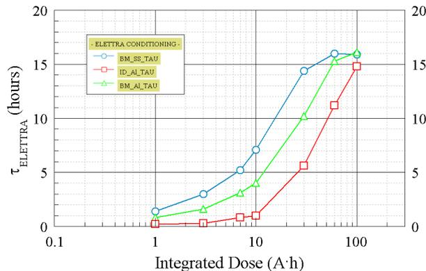
Figure 3: Elettra: tau versus integrated beam dose. BM\_SS: bending magnet stainless steel chamber; ID\_Al: ID aluminum chamber; BM\_AL: bending magnet aluminum chamber.
