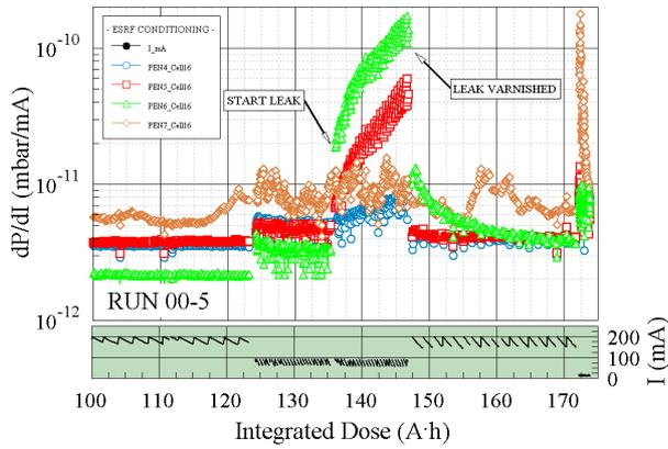
Figure 6: ESRF: corrosion leak, developing in cell 16.
