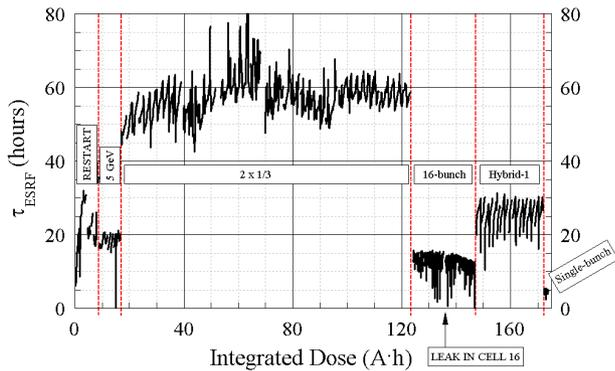
Figure 2: ESRF: beam lifetime evolution for Run 00-5.
