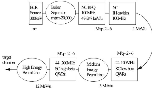
Fig. 1. Schematic diagram for acceleration of high-charge-state RIBs.
