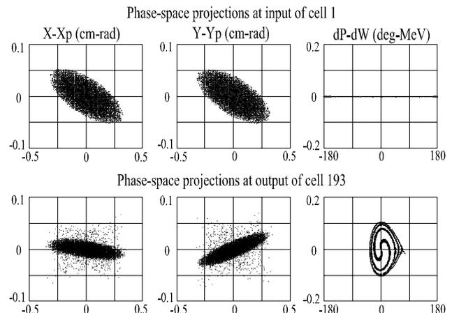
Fig. 2: Phase-space projections of beams injected into and exiting from the RFQ.
