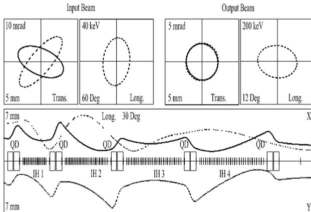
Fig. 3: Beam envelope through the IH linac
