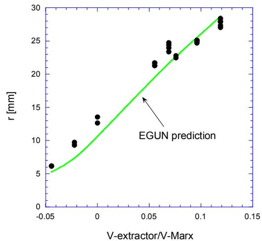
Figure 5. RMS beam sizes  $2\langle x^2 \rangle^{1/2}$  and  $2\langle y^2 \rangle^{1/2}$  for measured beam profiles, compared to EGUN predictions.
