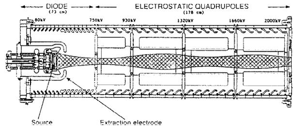
Figure 1. Cross sectional view of the Injector.
