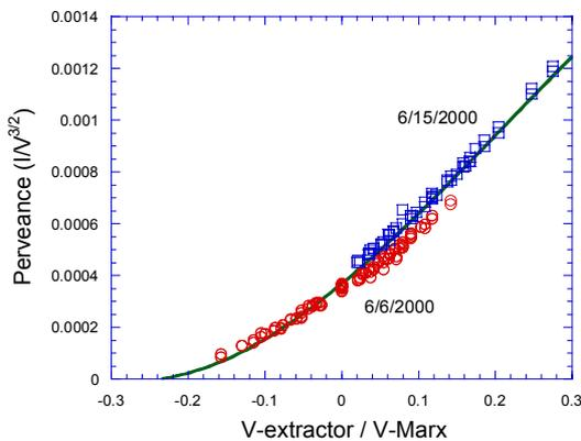
Figure 3. Comparison between measured and predicted (EGUN) beam current in the diode for the 10-cm diameter aluminosilicate source. Dates of measurements are indicated.
