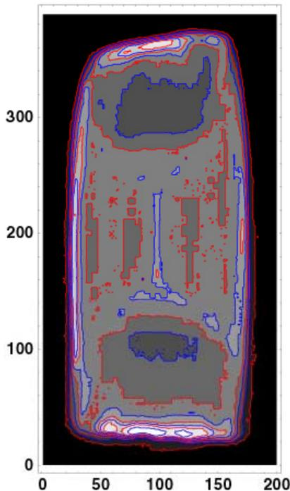
Figure 6. Contour plots of beam intensity from a Kapton film exposed by the beam, showing a raised rim and a rectangular shape. Intensity, indicated by the grayscale, is lowest for black and greatest for white. The internal structure in the image is due to an after-pulse, not the main beam pulse. The beam dimensions are roughly 5 cm x 10 cm. The scale is in pixels; each pixel is 25  $\mu\text{m}$  in size.
