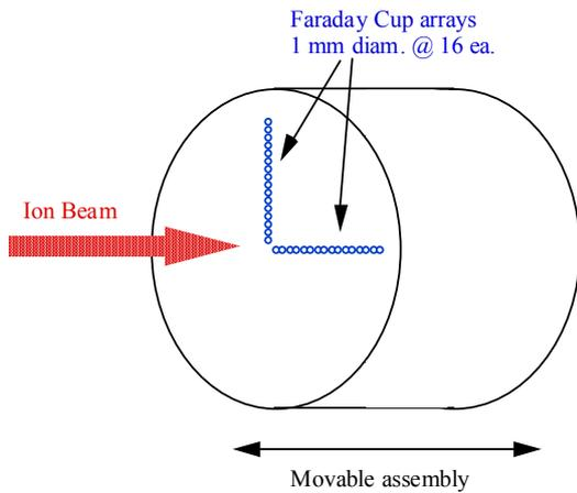
Figure 2. Schematic diagram of the 32-channel Faraday cup array.
