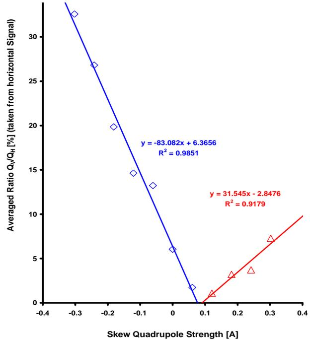
Figure 4: Linear Coupling compensation.
