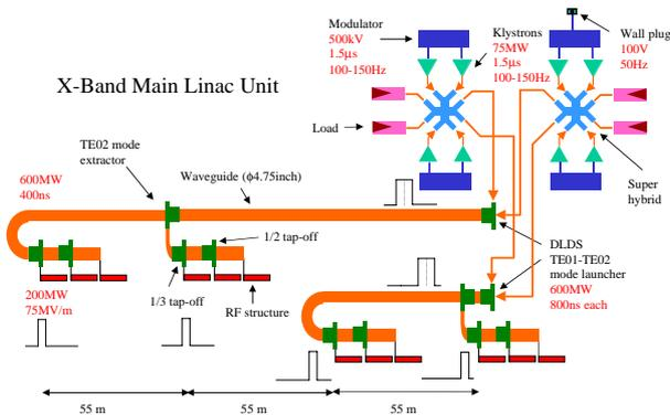
Figure 2: Schematic view of  $TE_{01}/TE_{02}$  2x2 DLDS
