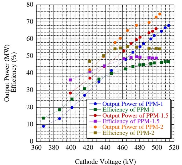
Figure 1: Output power and efficiency vs. cathode voltage at PPM-1, PPM-1.5 and PPM-2 klystrons
