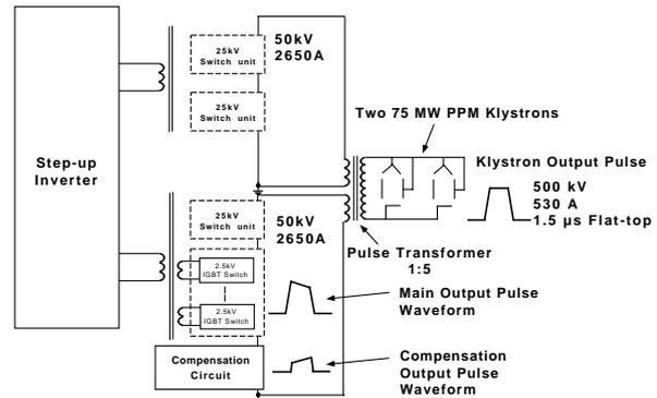
Figure 3: Diagram of the IGBT modulator.
