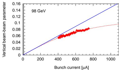
Figure 4: Vertical beam-beam parameter versus bunch current. The data is compared to the not beam-beam limited case and a fit [10].
