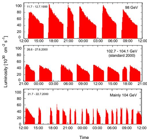
Figure 3: Instantaneous luminosity in LEP for three different days in 1999 and 2000. The different modes of operation for 98 GeV, 102.7 to 104.1 GeV (standard running in 2000) and mainly 104 GeV are clearly visible.
