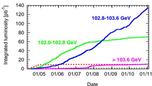
Figure 1: Luminosity production in 2000. The three ranges correspond to 2, 1 and 0 klystrons margin (right hand numbers, from top to bottom).
