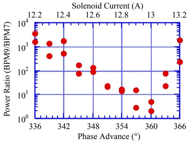
Figure 5. Spectral peak power as function of phase advance.
