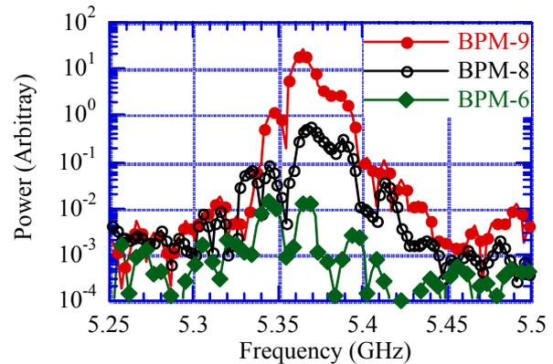
Figure 4. FFT Power Spectrum for 6<sup>th</sup>, 8<sup>th</sup>, and 9<sup>th</sup> BPM's.
