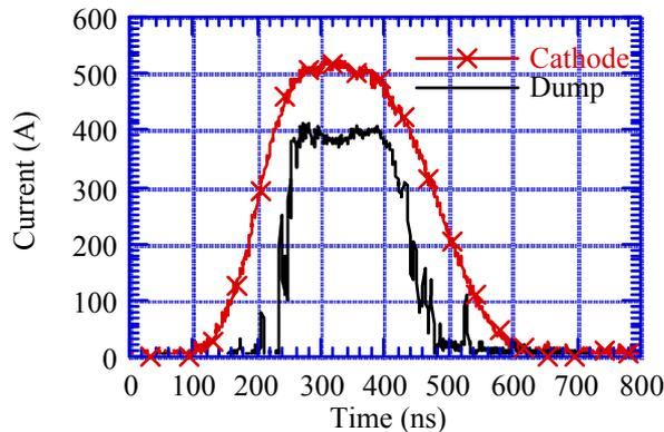
Figure 2. Typical Cathode and Dump current pulses.
