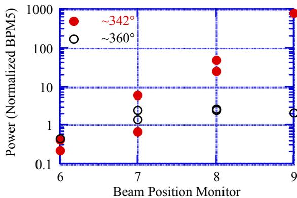
Figure 6. Spectral peak power as function of BPM for two different betatron phase advances.
