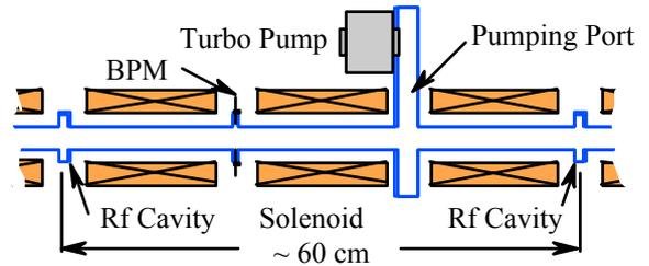
Figure 3. Repeating beamline section in BNS experiment. frequency below 500 MHz for display on a digital scope. The digitized traces were then down loaded to a computer and Fourier transformed to yield the power spectrum. Figure 4 shows examples of the resulting power spectra. In the following figures, power refers to the peak spectral power associated with the 5.36 GHz transverse mode.
