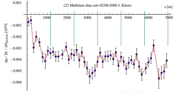
Figure 6: Change of the accumulated vertical phase advance around the SPS ring with bunch intensity [7].
