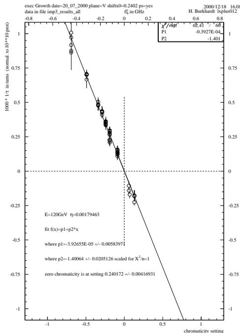
Figure 5: Growth rate of vertical head-tail mode (in units of  $10^{-3} \text{ turns}^{-1}$ ) measured as function of chromaticity  $\xi$  at 120 GeV on 19/07/2000.
