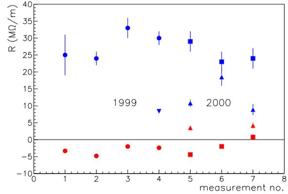
Figure 4: Impedance values  $R_{\perp}^{\Delta Q}$ ,  $x(y)$  inferred from all measurements in 1999 (first 4) and 2000 (the last 3), by fitting to a broadband resonator with resonant frequency  $\omega_r/2\pi = 1.3$  GHz and quality factor  $Q = 1$  [3]. Triangles are the  $R_{\perp}$  values obtained from the growth rate measurements; squares and circles represent  $R_{\perp}^{\Delta Q}$  inferred from the coherent tune shift. The 6th measurement was performed at 120 GeV, all others at 26 GeV.
