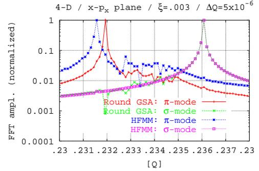
Figure 4: The spectra of the  $\pi_x$ - and  $\sigma_x$ -mode computed with BBDeMo2D with  $51^4$  particles in the round GSA (red, green) and with  $45^4$  particles in the HFMM approach (blue, purple).
