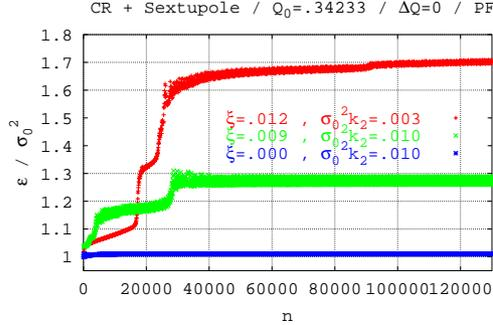
Figure 3: Emittance growth with beam-beam and Sextupole. PF with  $401 \times 401$  over  $\pm 6\sigma_0$ .  $\sigma_0^2 k_2$  is the normalized sextupole strength.
