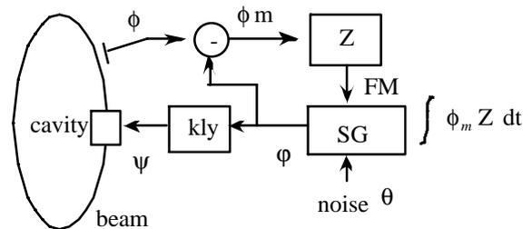
Figure 1: Beam phase and RF system.
