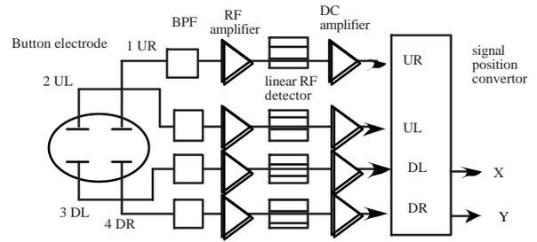
Figure 3: Set-up for the measurement of beam position.
