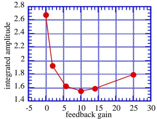
Figure 7: The integrated value of the spectrum as a function of the feedback gain.
