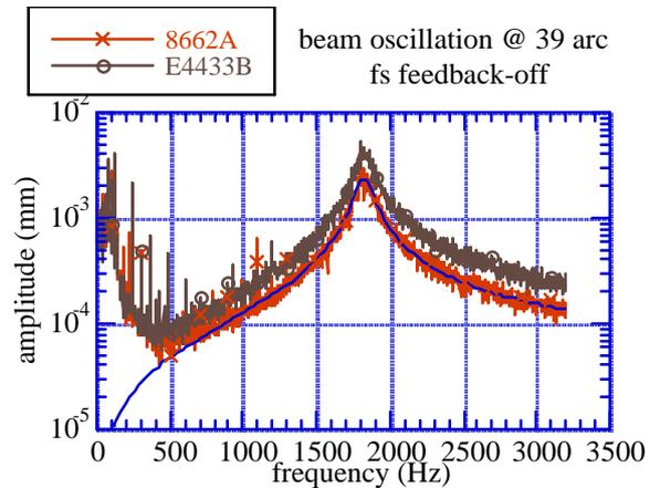
Figure 4: Beam position spectrum measured at 39 arc.
