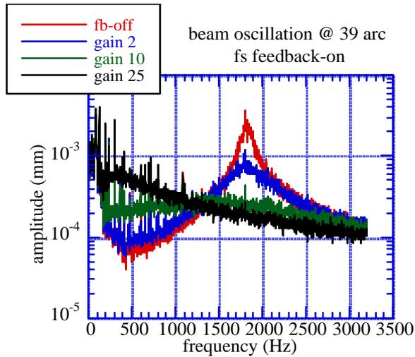
Figure 5: The measured beam position spectrum.
