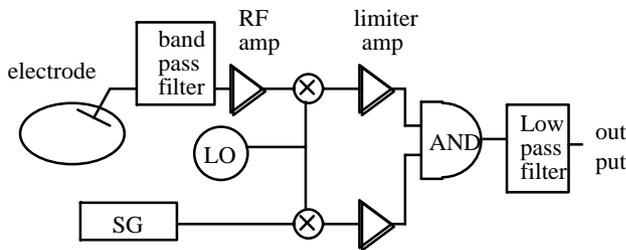
Figure 2: Set-up for beam phase measurement.
