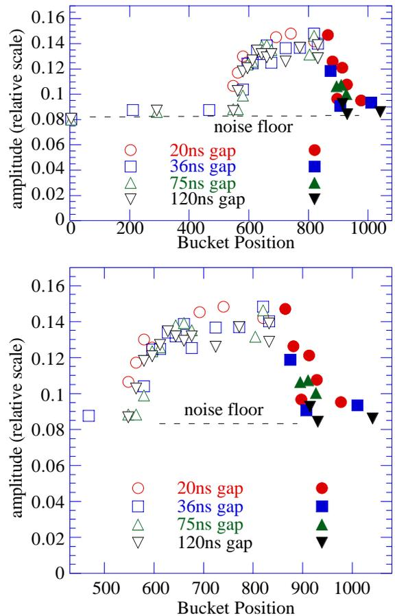
Figure 4. Betatron amplitude distribution in two bunch train with different gap width between them. Marks filled inside is the data for the 2nd train. Upper graphs shows The motion of whole bunches and lower graph shows expanded area where betatron amplitude was observed.
