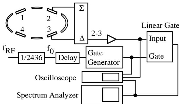
Figure 2: Experimental setup for measurement of position dependence of betatron oscillation amplitude. RF signal is divided to revolution frequency for a gate signal.
