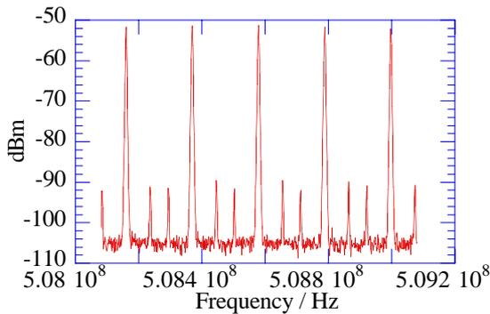
Figure 3: Typical data taken by spectrum analyzer. Higher peaks are harmonics of revolution frequency and lower peaks are vertical betatron sideband. Harmonic signal of
