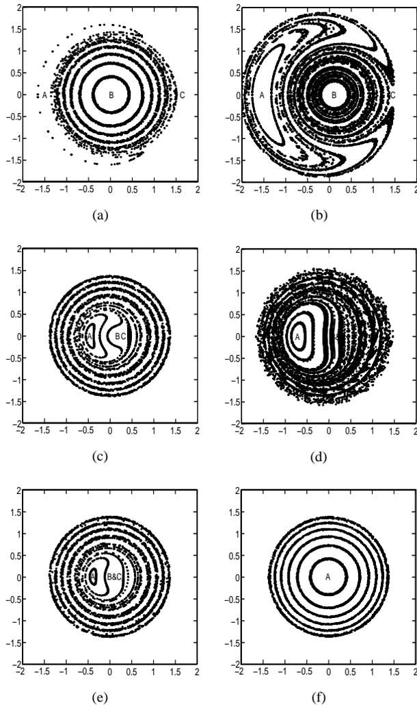
Figure 1: Phase space tracking of the RF phase modulation for (a)  $a_m = 0.003$  at *may18am*, (b)  $a_m = 0.030$  at *may18am*, (c)  $a_m = 0.003$  at *may18pm*, (d)  $a_m = 0.030$  at *may18pm*, (e) the bifurcation frequency at *may18pm*, and (f) *jun06am* conditions. Here, the horizontal and the vertical axes mean  $\sqrt{2\tilde{J}} \cos(\tilde{\psi} - \nu_m \theta)$  and  $\sqrt{2\tilde{J}} \sin(\tilde{\psi} - \nu_m \theta)$ , respectively.
