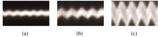
Figure 2: Streak camera images of the beam motion when the bunch length beating is generated due to a single 5.244 kHz RF noise driven phase modulation. The maximum horizontal time scale is 1 ms and the vertical time scale which means the bunch length is same for three cases.
