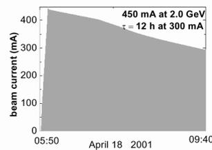
Figure 6: Stored beam current of 450 mA at 2.0 GeV.
