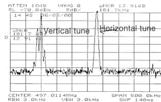
Figure 5: Beam spectrum shows increased magnitude and side-bands in vertical tune when number of bunches is 468.
