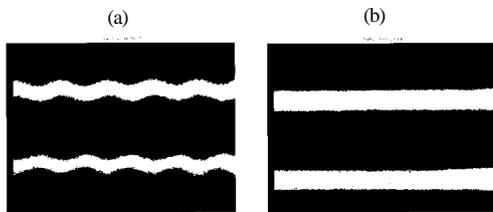
Figure 1: Beam oscillations at 2.5 GeV that are observed in streak camera. (a) the number of bunches is 468,  $\nu_x=14.26$  and  $\nu_y=8.15$ . (b) the number of bunches is 400,  $\nu_x=14.28$  and  $\nu_y=8.18$ . Beam currents in (a) and (b) are 115 mA and 110 mA, respectively.
