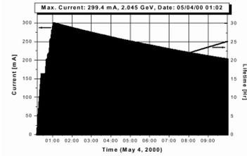
Figure 3: Stored beam current of 300 mA at 2.0 GeV.
