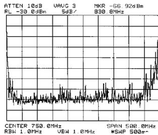
Figure 2: Beam spectrum on spectrum analyzer in the beam current of 193 mA at 2.5 GeV. The spectrum shows frequency band between 500 MHz and 1 GHz.
