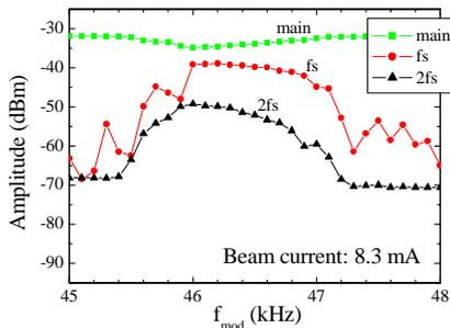
Figure 5: Beam response when the phase-modulation frequency was swept upward while keeping its amplitude.
