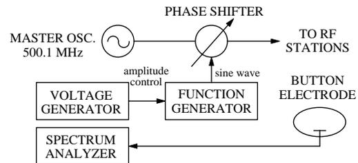
Figure 1: Experimental setup.
