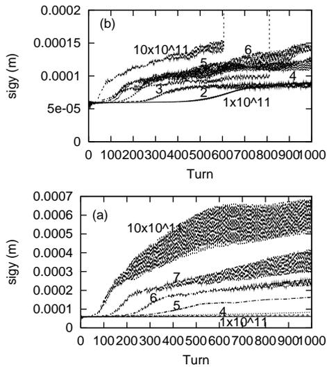
Figure 2: Beam size evolution for various cloud densities.
