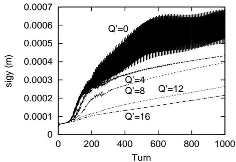
Figure 3: Chromaticity dependence of instability for  $\rho = 10^{12} m^{-3}$ .
