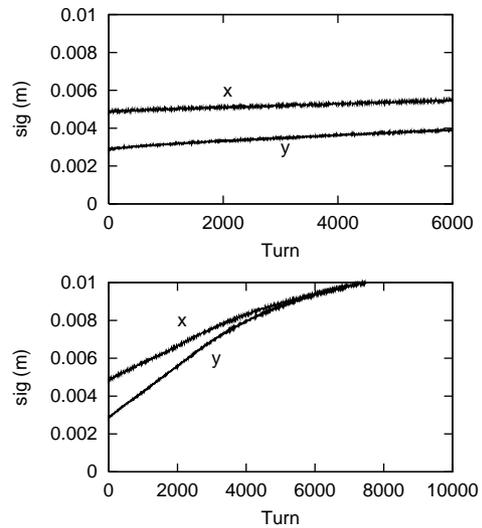
Figure 4: Beam size evolution of SPS instability.
