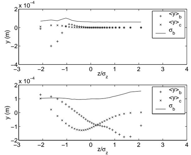
Figure 1: Beam dipole moment and size, and cloud dipole moment for without and with synchrotron oscillation, (a)  $\nu_s = 0$  (b)  $\nu_s = 0.015$ . Head part of beam corresponds to positive  $z$ .
