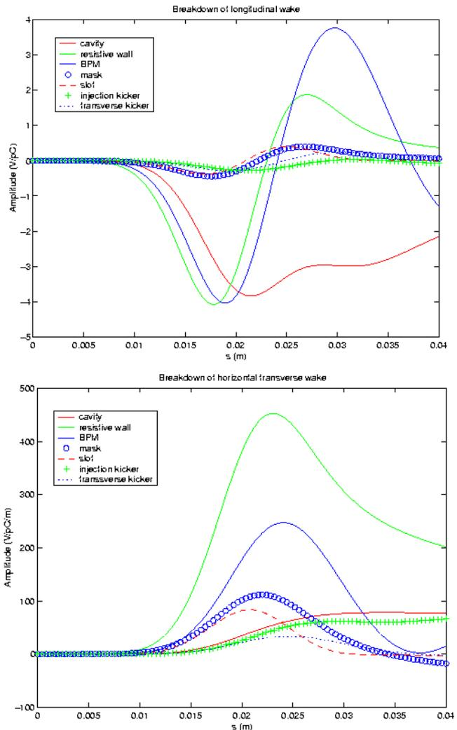
Figure 1. Short-range wakefields, longitudinal (top), horizontal (bottom).
