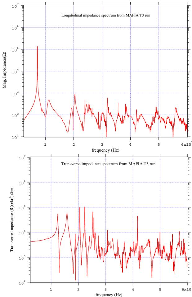
Figure 2. Long-range cavity wakefields, longitudinal (top), transverse (bottom).
