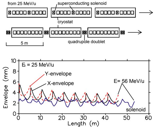
Figure 3: Upper: Two different layouts of focusing elements downstream of the charge stripping section (25 MeV/u) using either superconducting solenoids or normal-conducting quadrupole doublets. The layouts of the elements and cryostats are generated from the input table used for the beam dynamics calculations. Lower: The beam envelopes for a normalized rms emittance of  $0.15 \pi$  mm-mrad.
