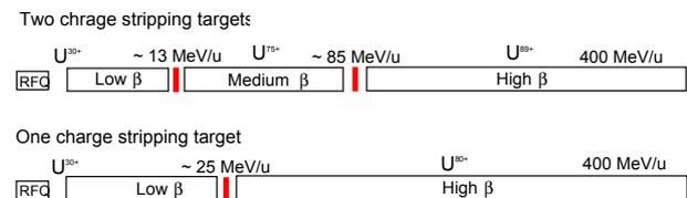
Figure 1: Layouts of heavy-ion driver linacs from the RFQ linac in the single and double charge stripping cases for very heavy ions.
