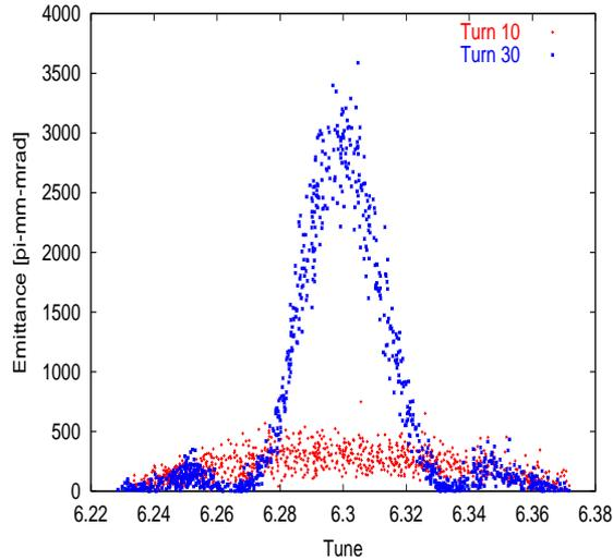
Figure 1: Emittance vs. Tune after 10 turns and 30 turns of the beam, with the kicker firing on resonance with  $\nu = 6.3$ .
