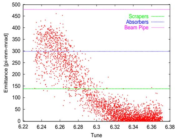
Figure 4: Emittance vs. Tune after 10 turns. Note that because of the phase dependence of the betatron motion, some particles climb to very high emittances before making contact with the collimation system.
