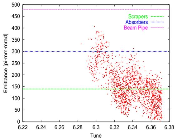
Figure 5: Emittance vs. Tune after 30 turns. In this example, all of the particles are absorbed by turn 40.
