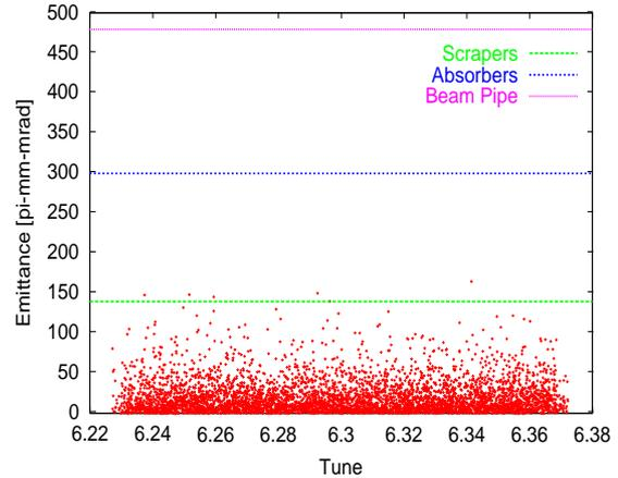
Figure 3: Emittance vs. Tune before kicking for a distribution with  $\delta = \frac{\Delta P}{P} = 0.01$ .
