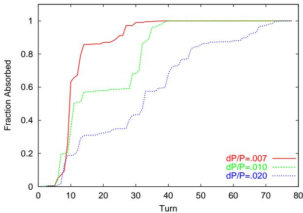
Figure 2: Fraction of particles absorbed per turn for momentum deviations corresponding to the anticipated momentum spread (0.007), the RF momentum aperture (0.01), and the dynamic aperture (0.02).
