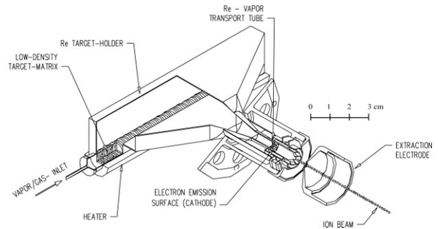
Figure 6: High vacuum conductivity target/vapor transport/ion source system for fast effusive-flow.
