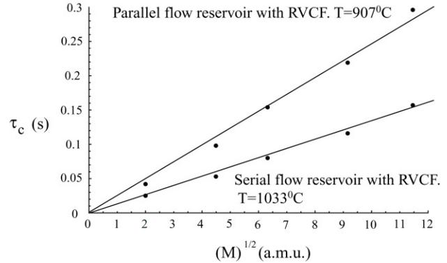
Figure 5: Measured characteristic effusive-flow times,  $\tau_c$ , for noble gases versus  $(M)^{1/2}$ . Experiment:  $\bullet$ ; Theory —.
