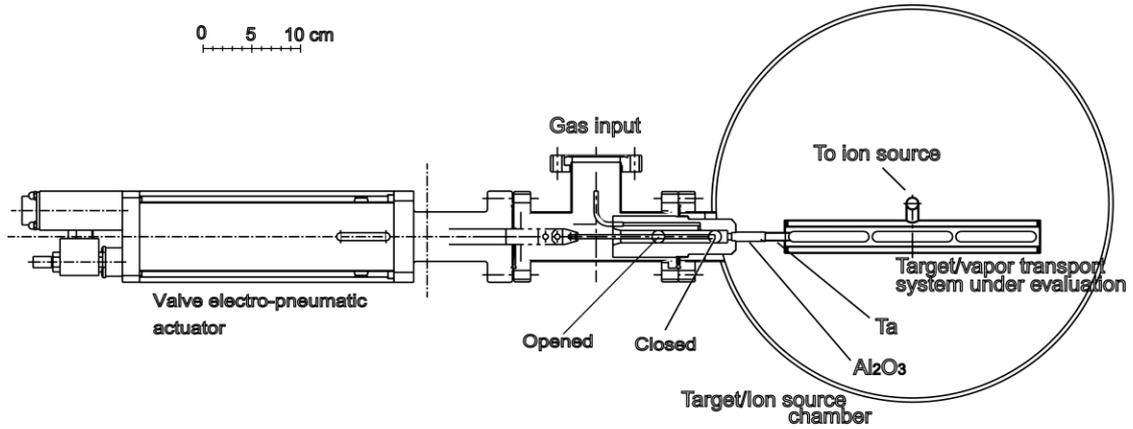
Figure 1: Schematic drawing of the fast closing valve, gas input system on the target/ion source chamber.
