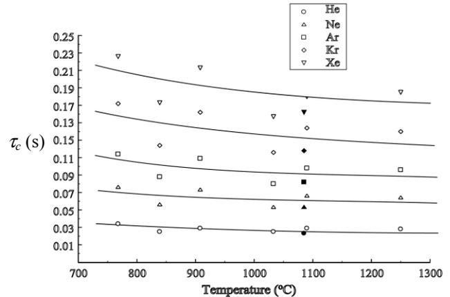
Figure 3: Characteristic times,  $\tau_c$ , for noble gases versus temperature,  $T$ , of the target material reservoir with (open symbols) and without RVCF material (solid symbols).
