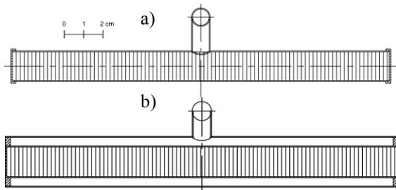
Figure 2: a) The serial-flow and, b) parallel-flow reservoirs to be characterized.
