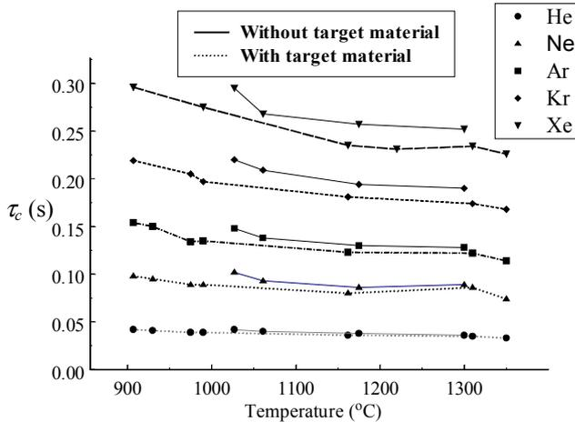
Figure 4: Characteristic time,  $\tau_c$ , for noble gases versus target material reservoir temperature,  $T$ , with and without RVCF material.
