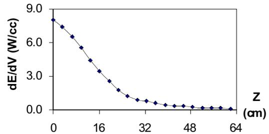
Fig. 2: Beam power density deposited by a parallel incidence, 1 GeV, 1 μA proton beam, along the beam axis of a UC<sub>2</sub> target. Density: 2.5 g/cc; Length: 65 cm; Beam Diameter: 0.5 cm.
