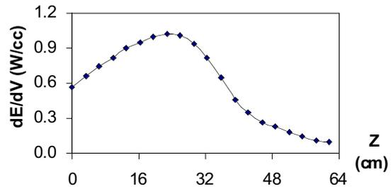
Fig. 3: Beam power density deposited by a converging incidence, 1 GeV, 1 μA proton beam along the axis of a UC<sub>2</sub> target. Density: 2.5 g/cc; Length: 65 cm; Incident beam spot diameter: 2 cm.
