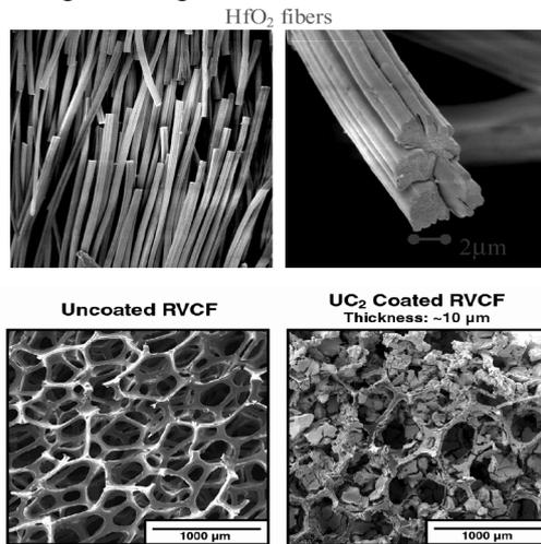
Fig. 1: SEMs of HfO<sub>2</sub> (upper) and UC<sub>2</sub> (lower) targets
