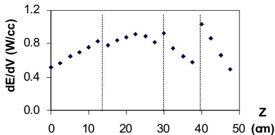
Fig. 4: Beam power density for a 1 GeV convergent proton beam along the axis of a  $UC_2$  target with 4 different densities (2.49 g/cc, 2.0 g/cc, 2.52 g/cc, and 6.0 g/cc) ordered from beam entrance to exit in four sections, as indicated. Incident beam: spot size  $\sim 2.2$  cm; Intensity:  $1 \mu A$ .
