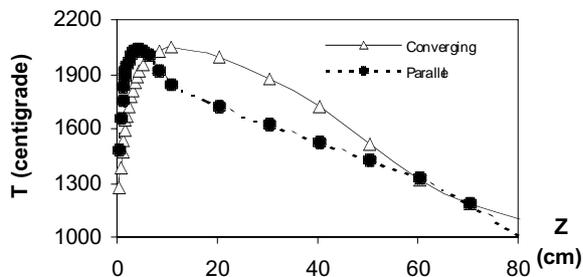
Fig. 5: Temperature distributions in  $UC_2$  targets irradiated with 1 GeV, 20 kW parallel and, 30 kW convergent incidence proton beams. Density: 2 g/cc; Length: 85 cm; Diameter 4 cm.
