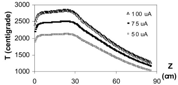
Fig. 6: Temperature in a tantalum target irradiated with 1 GeV, 50 kW, 75 kW, and 100 kW, converging proton beams. Density: 2.1 g/cc; Length 85 cm; Diameter 4 cm.
