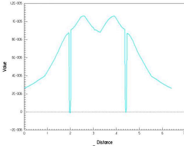
Figure 1: Magnetic field (per Ampere) profile calculated by MAXWELL.
