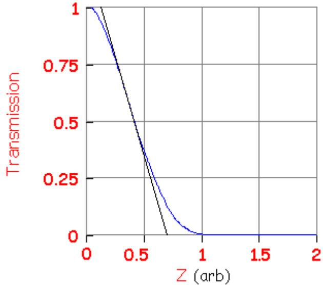
Figure 2. As Fig. 1, the resulting transmission of electrons through a thickness of material (curve). The straight line is an extrapolation of the linear part of the curve.
