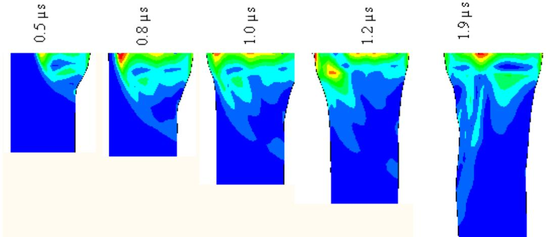
Figure 3. Stress pattern sequence produced in thin tantalum foil due to the passage of a swept electron beam over the width (travelling from the bottom of the foil to the top).
