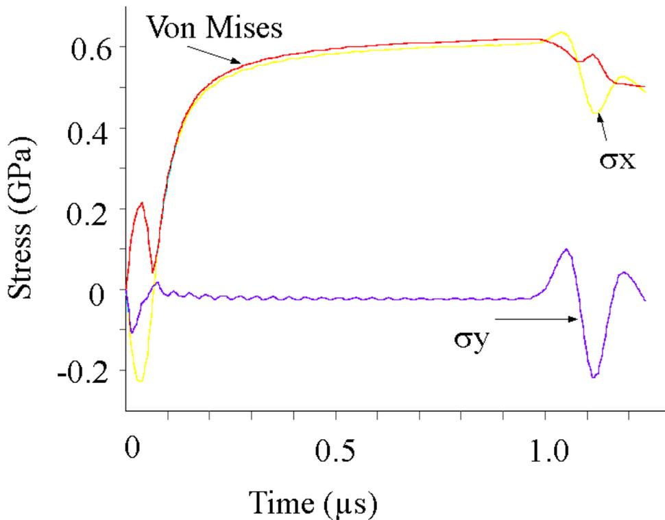
Figure 4. Surface stress levels in the foils as a function of time.
