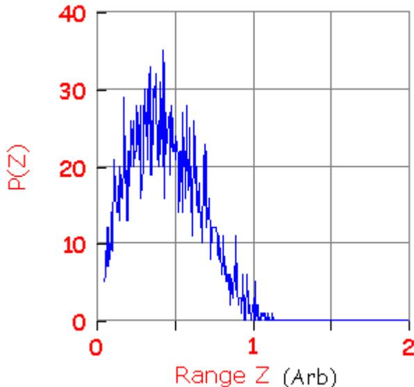
Figure1. Monte Carlo modelling of the Energy Deposition of a beam of 100 keV electrons in Tantalum.
