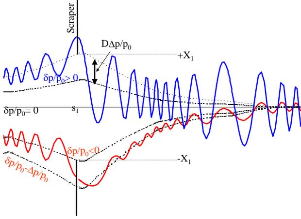
Figure 1: Schematic view of the use of thin scrapers for momentum collimation. After the traversal of the scraper, the closed orbit decreases a factor  $p_{loss}/p_0$ . The betatron oscillation around the closed orbit is enhanced for  $\delta > 0$  while for  $\delta < 0$  we have cooling.
