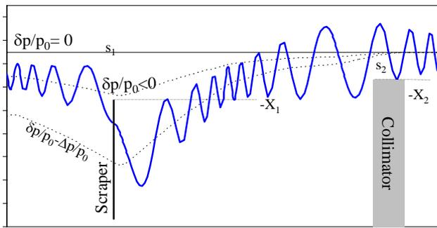
Figure 2: Absorption of the momentum halo by a secondary absorber after interaction with the striper.
