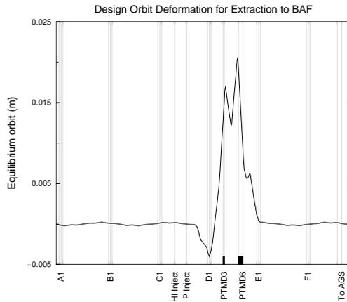
Figure 2: Orbit deformation at the thin and thick septa.
