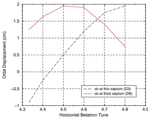
Figure 5: Displacement at thin and thick septa versus tune, for a 2 mrad kick from the F3 kicker, at  $B\rho=17$  Tm.
