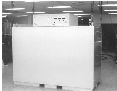
**Figure 5. 140-kV, 20 A buck regulator installed at CPI.**
