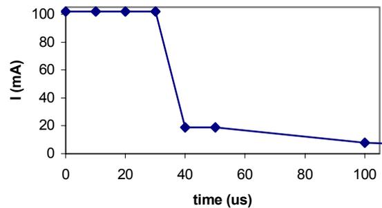
Figure 2. Beam current vs. RF interruption. An interruption of up to 30  $\mu$ s can be sustained without beam loss.
