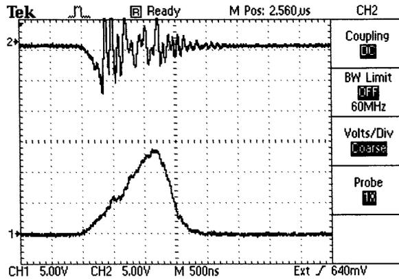
**Figure 3. Left: Opening switch delivered to CPI. Right: Waveforms of a deliberate short. Upper trace, voltage, 50kV/division; lower trace, current, 250 A/division.**
