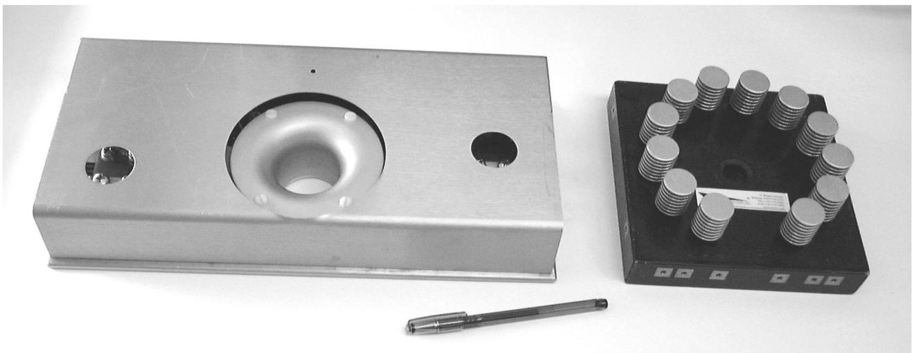
**Figure 4. Switch modules. Left: 3kV high-current (65A DC, 750A pulsed). Right: 6kV low-cost (25A DC, 250A pulsed).**
