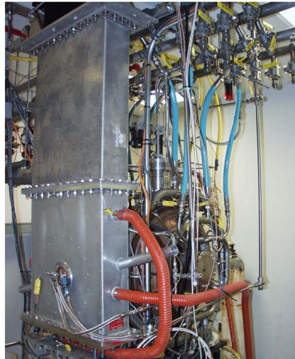
Figure 4: rf test cavity assembly.
