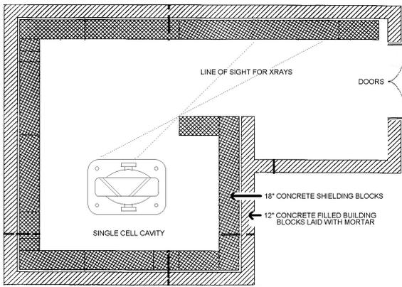
Figure 2: Test bunker top view.
