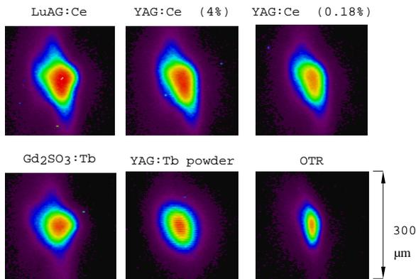
Figure 3: Beam images taken consecutively with the six different diagnostics under the stable experimental conditions (the charge  $Q \sim 500$  pC).
