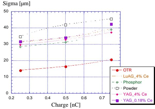
Figure 4: Electron beam horizontal spot size as a function of charge, measured with the scintillating diagnostics and the OTR.
