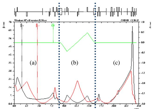
Figure 1: Evolution of the electron beam  $\beta$ -functions and a dispersion function along (a) post linac focusing channel; (b) dispersion section; (c) beam line 1 focusing optics.
