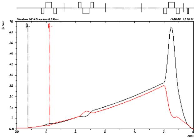
Figure 2: Beam optics layout including a permanent quadrupoles cell at the final focus.
