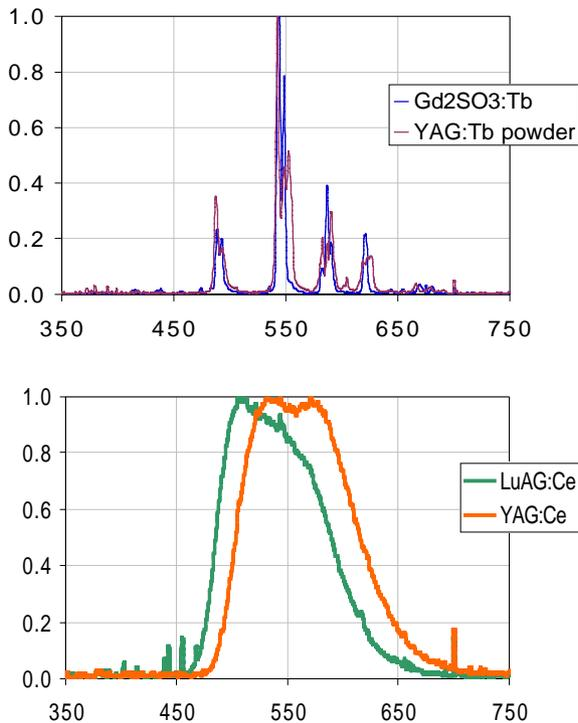
Figure 5: Spectral profiles of Tb doped and Ce scintillators emission respectively, under the electron beam excitation. Small dip at 550 nm in the YAG:Ce emission profile was very distinct and repeatable.
