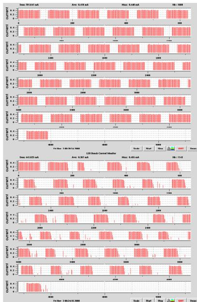
Figure 4: Special filling pattern before (upper) and after (lower) switching off/on the feedback.
