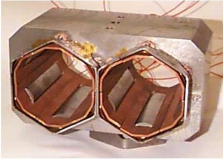
Figure 5: The sextupole cold mass. End covers are visible.
