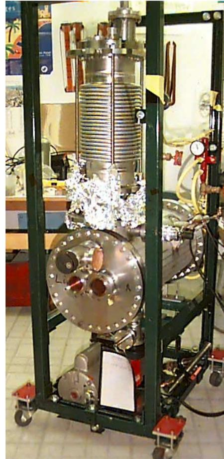
Figure 1: Dual bore quadrupole magnet installed in a cryostat for cryogenic test. In a vertical bellow there are joints allowing the He filling from standard Dewar. Diameter of the main body is  $\cong$  10 inches.
