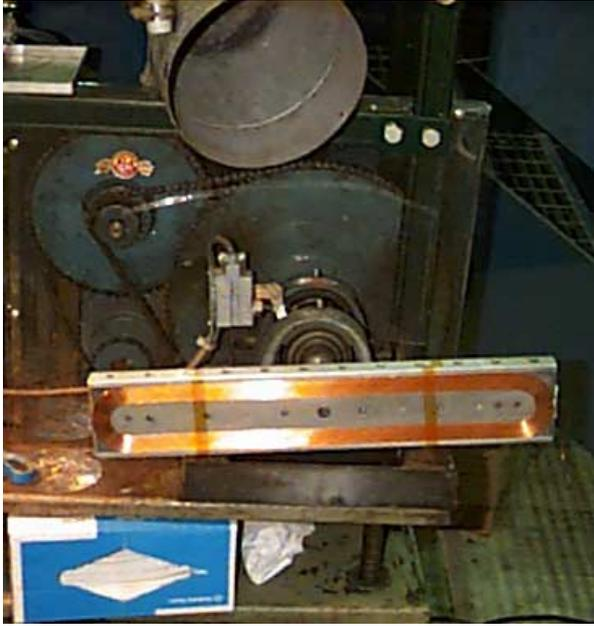
Figure 5: The winding fixture installed in the winding machine shown. The top cover removed, so the coil could be visible. SC wire is coming vertically from the spool located at the top of machine. Tension of the wire regulated with special brake.
