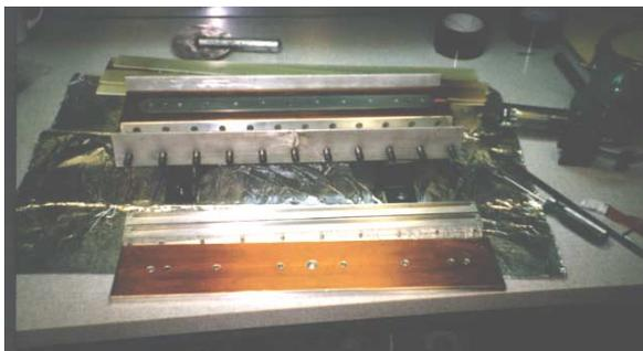
Figure 2: The winding set. At the top of the picture the pizza cutter style roller is visible.
