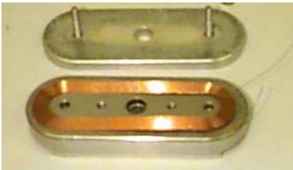
Figure 6: The winding fixture for sextupole coil. Basically it is a scaled version of the fixture used for quadrupole coil winding.
