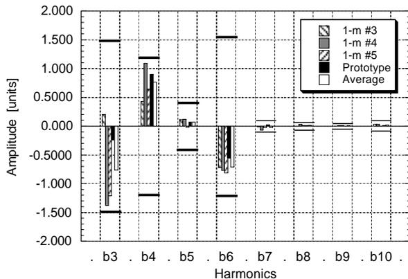
Fig. 6. Measured harmonics in the 1-m models and the prototype. The top and bottom bars indicate envelope of the reference harmonics including the systematic errors, uncertainty, and standard deviation.
