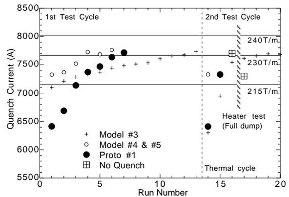
Fig. 5. Training characteristics of MQXA 1-m models and a prototype. 1-m models #4-#5 tested in series connection.
