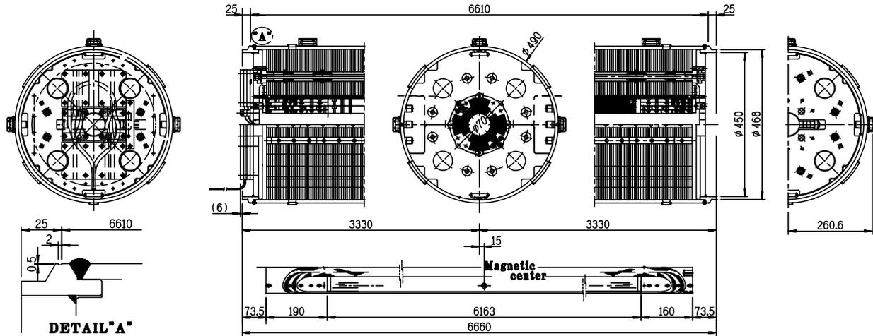
Fig. 3. Cross sections of the LHC low- $\beta$  quadrupole, MQXA, being developed at KEK.
