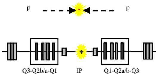
Fig. 1. Schematic layout of LHC low- $\beta$  inner triplet.
