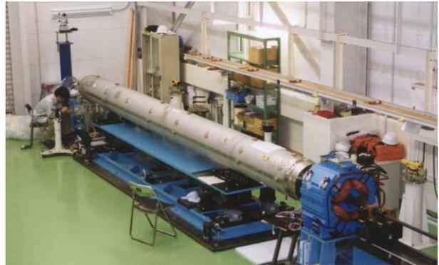
Fig. 2. A prototype of LHC low- $\beta$  quadrupole (MQXA) in field measurement at room temperature at KEK.
