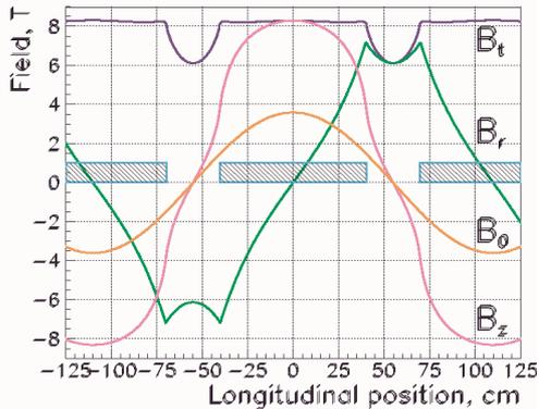
Fig.2. Magnetic field distribution for solenoid with  $L=0.8$  m and  $d=175$  mm.
