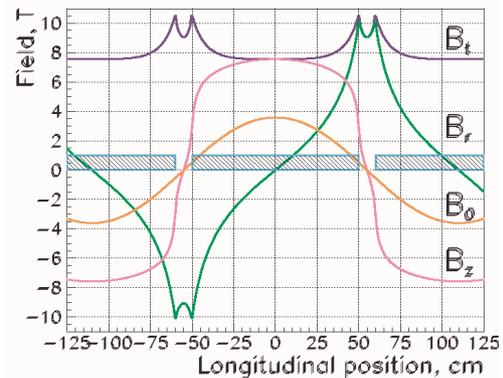
Fig.1. Magnetic field distribution in the cooling channel for solenoid length  $L=1$  m.
